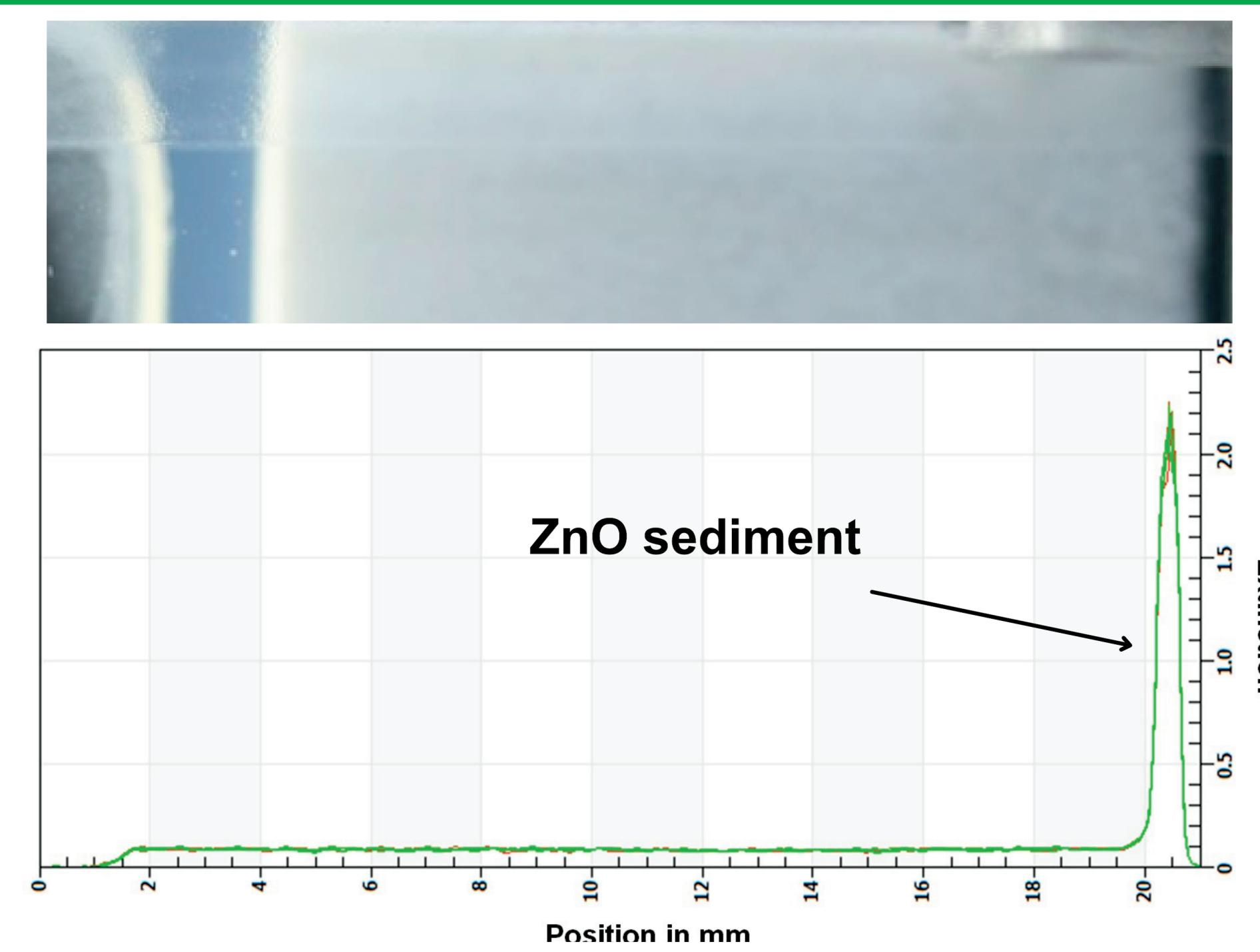
Pigment (ZnO) segregation within opaque sun protection cream: Accelerated separation for 120 min at RCA = 2300 g (LUMiSizer) and attenuation profiling (LUMiReader X-Ray)
