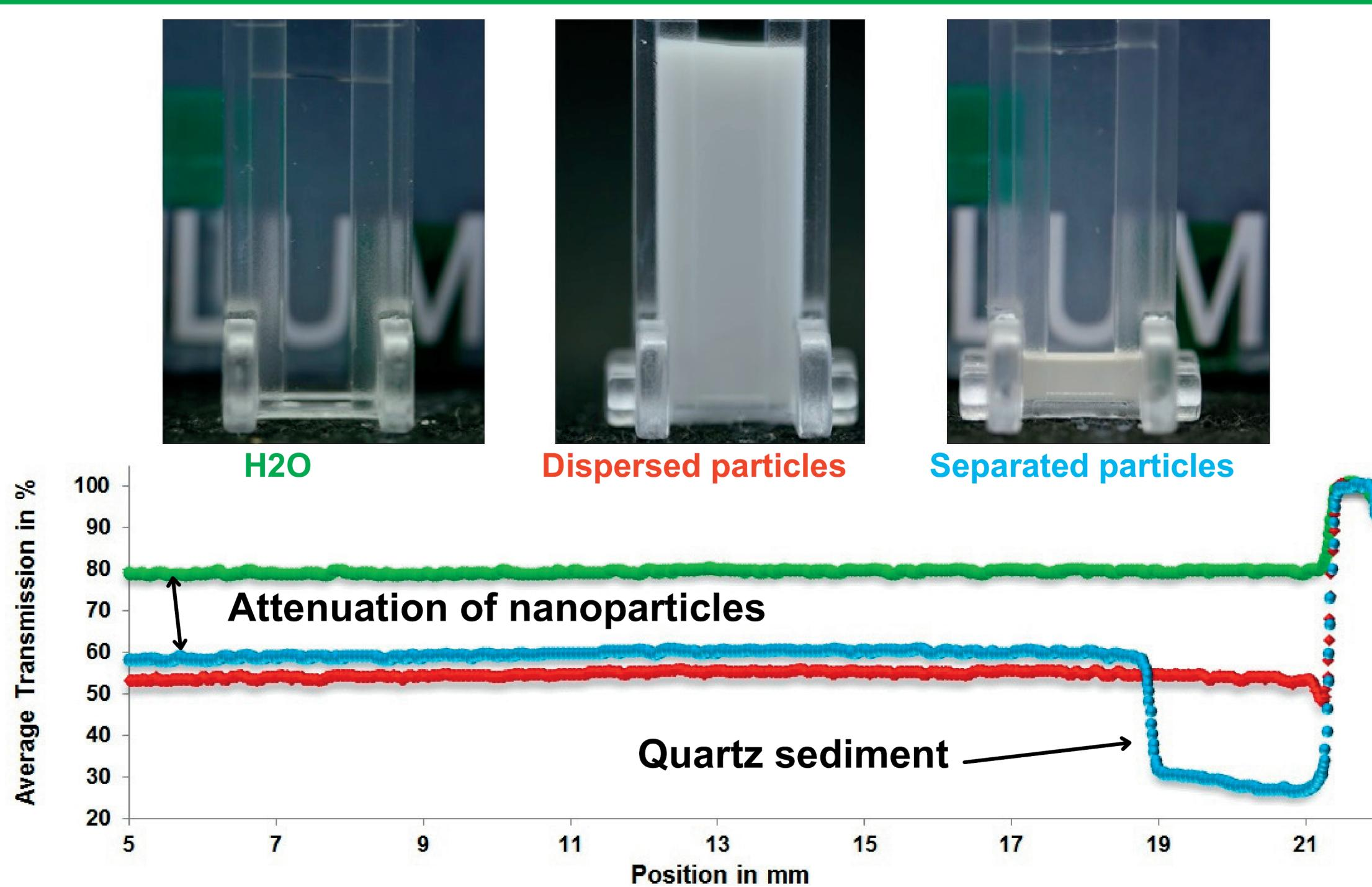
Detection of nanoparticles in supernatant of suspension consisting of 10 % Quartz + 30 % w/w Koestrosol® (15 nm) in water after accelerated separation (10 min at 25°C, RCA = 2300 g)
