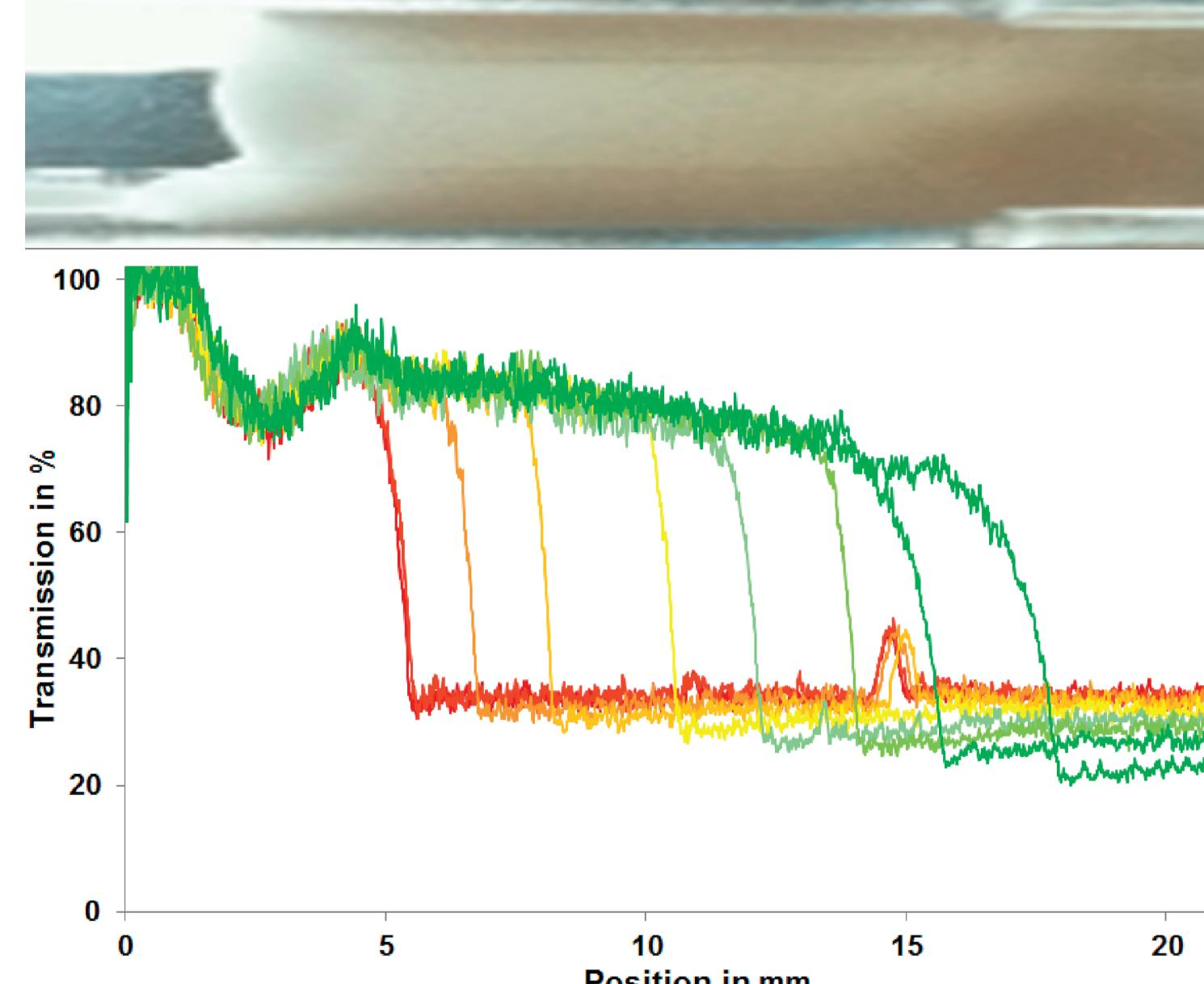
X-ray profiles allow to trace in real-time kinetics of invisible processes. Separation of a filler inside an adhesive matrix (earth gravity). Right comparison of 3 adhesive formulations.
