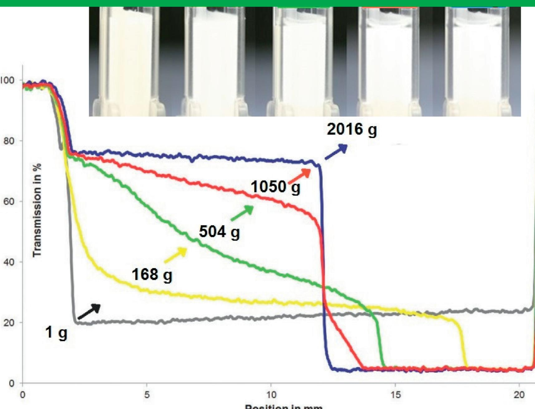
Concentration profiling of filler dispersed in polymer (61% m/m) with LUMiReader X-Ray after accelerated separation for 60 min at 25°C, RCA = 168 g to 2016 g
