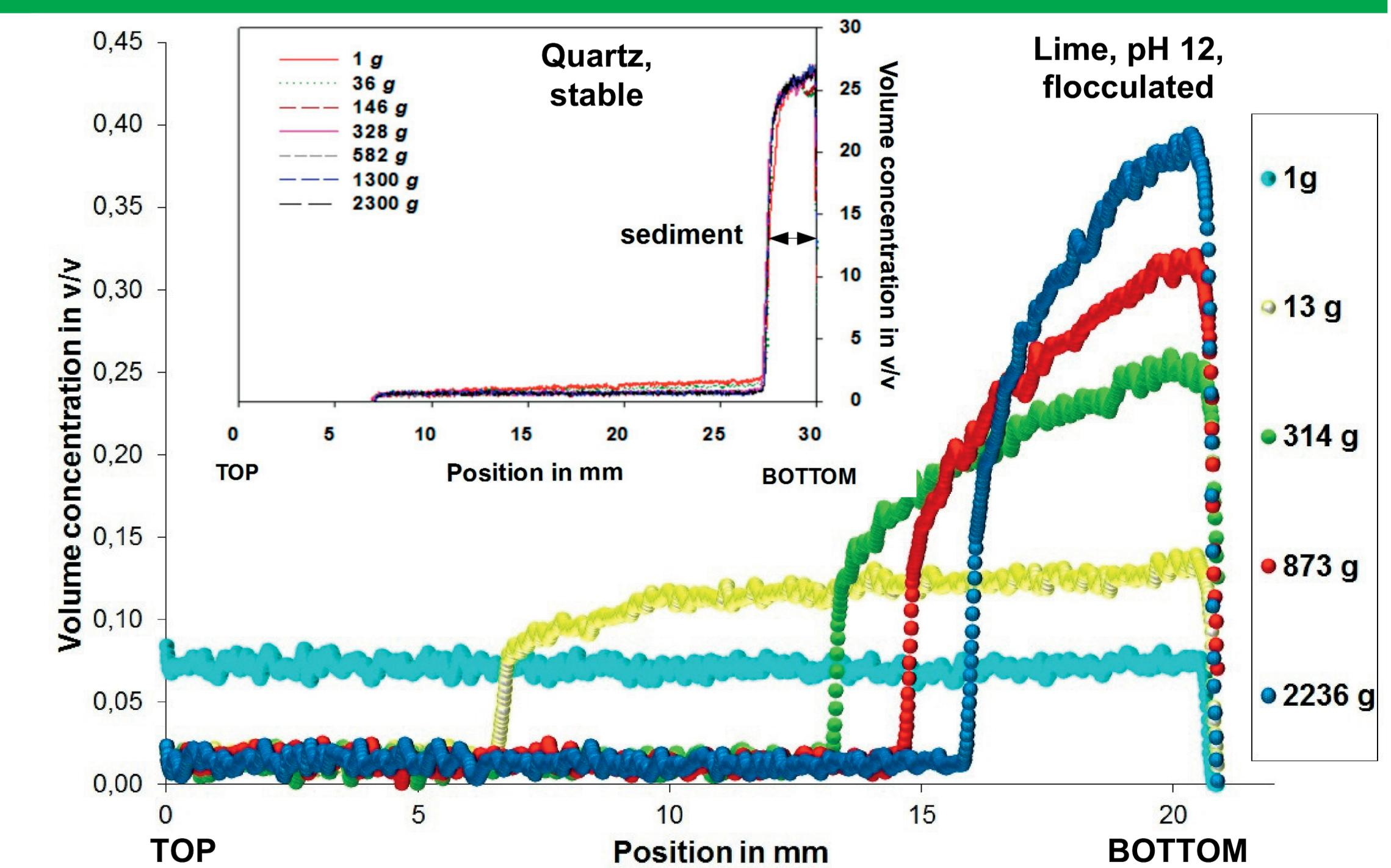
Sediment packing profiling by X-ray after consolidation (different centrifugal forces and particle interaction)
